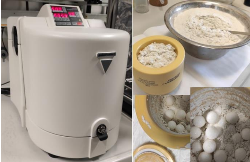
Figure 1. Planetary ball mill „PULVERISETTE 6 classic line“ (left); loading of its grinding bowl with feather particles after centrifugal mill treatment and dry milling using 15 mm grinding balls (right)
